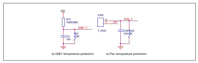
Figure 2-7 Over-Temperature Protection
